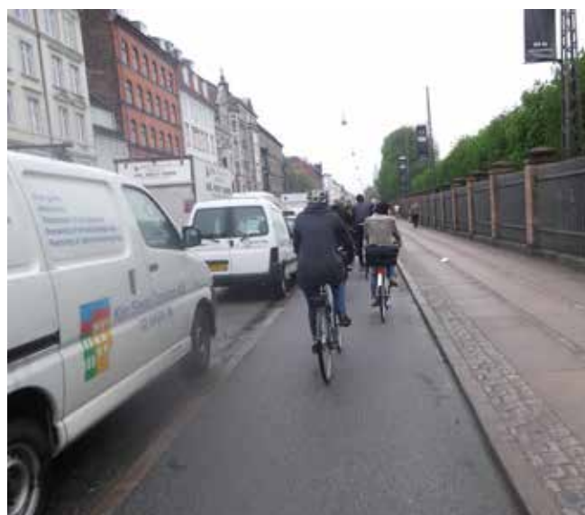
Copenhagen: the track is step-separated from the adjacent footway, and is also usually in visually different materials
