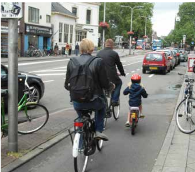
Utrecht - ahead cycle traffic from the nearside track has to cross right-turning general traffic approaching the stop-line
