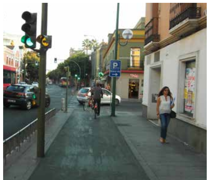
Seville - a flashing amber aspect reminds drivers to give way to crossing pedestrians and cyclists when making the turn
