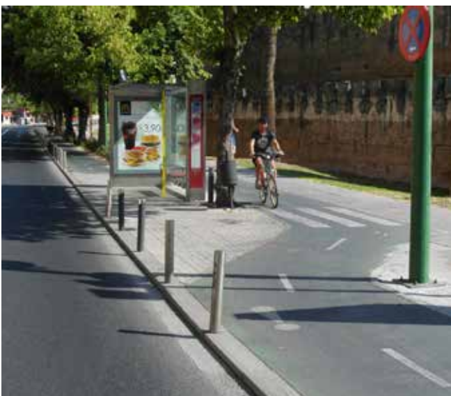
A typical bus stop bypass in Seville
