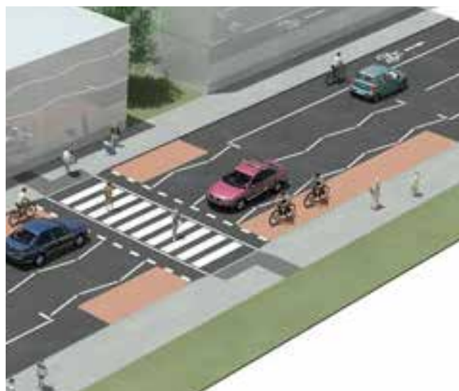
Irish National Cycle Manual: cycle lane markings through zebra zig-zags. Such arrangements should be readily permissible in the UK from 2015.
