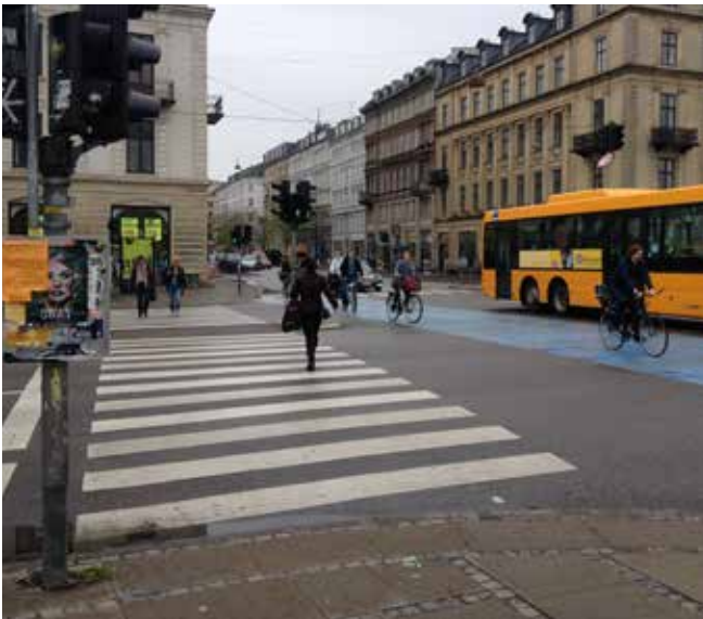
Copenhagen - Pedestrians & cyclists go on green with motor traffic required to give way on turns, so that...
