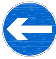
Diag No 606 Vehicular traffic must proceed in the direction indicated by the arrow
