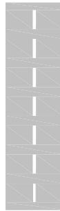
Diag No 1009 Marks the start of a cycle lane when laid diagonally across part of the carriageway.
