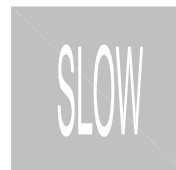
Diag No 1058.1 Marking used to alert cyclists to potential hazard ahead.
