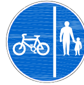
Diag No 957 Route comprising two ways, separated by the marking shown in Diag No. 1049 or 1049.1 or by physical means, for use by pedal cycles only and by pedestrians
