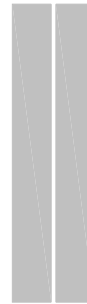
Diag No 1049 Line used to indicate boundary of mandatory with-flow cycle lane, or divide segregated cycle/pedestrian path
