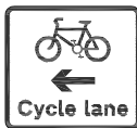
Diag No 962.1 Cycle lane on road at junction ahead or cycle track crossing road
