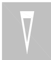
Diag No 1023 Give way marking (half size option for cycles used in conjunction with Diag No.1003)
