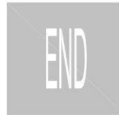
Diag No 1058 May be used to mark the end of a cycle facility, however positive marking and signing is normally sufficient.
