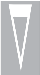
Warning of 'Give Way' just ahead
